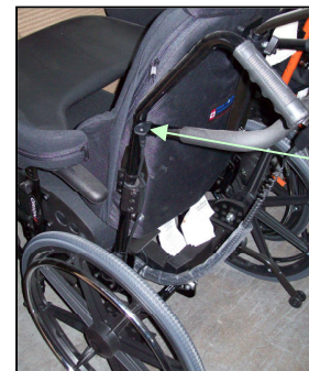
Cable extension for Battery/Control box (Item #15)
